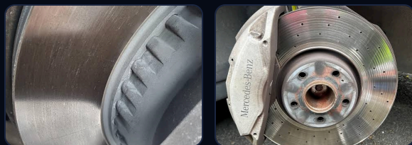
Left: a healthy rotor face. Right: a worn rotor with a lip at the edge.
